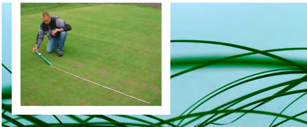
Research technician Trond Pettersen measures ball roll distance with a modified stimpmeter in Primo MAXX® trial at Landvik. Photo: Trygve S. Aamlid.
